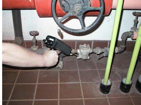
and is used as a predictive tool for steam trap monitoring. Ultrasonic testing permits the testing person to hear the internal operation of the steam trap; so the effectiveness of the steam trap operation can be determined.
